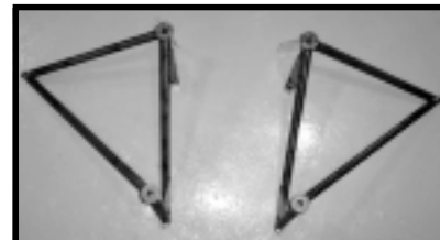
Above: KitFox Engine Mount Left: Avid Flyer Engine Mount
